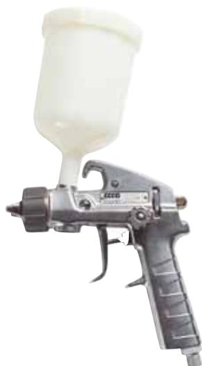
Gravity feed spray gun, where the sprayed material is supplied from a 0,5 litre paint cup. Paint channels in stainless steel for long life-time, also when spraying glaze or vitrous enamel. Fluid needles and nozzles in tungsten carbide is available.
