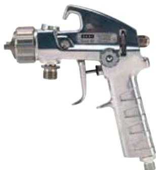
Pressure feed spray gun, with robust design and high quality components. The material is supplied from pressure pots, pumps or circulation system. Stainless Steel material channels as standard, tungsten carbide needle and nozzle available. High quality components and easy maintenance makes this gun ideal for the ceramic industry.
