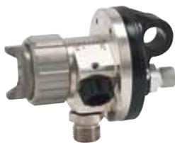
The Ecco 40DA is an automatic spray gun for spraying abrasive and other similar material (i.e. vitreous enamel). The gun has no paint needle. The material flow is accurately controlled by a diaphragm, sealing against a tungsten carbide seat. The gun is small and easy to install.
