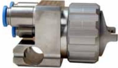
The Ecco 40FA is an automatic spray gun for spraying abrasive and other similar material (i.e. vitreous enamel). The gun has no paint needle. The material flow shall be controlled externally, paint nozzle in tungsten carbide for long lifetime. The gun is small and easy to install on a 13 mm beam. Atomizing air and fan air separately fed by external air supply.
